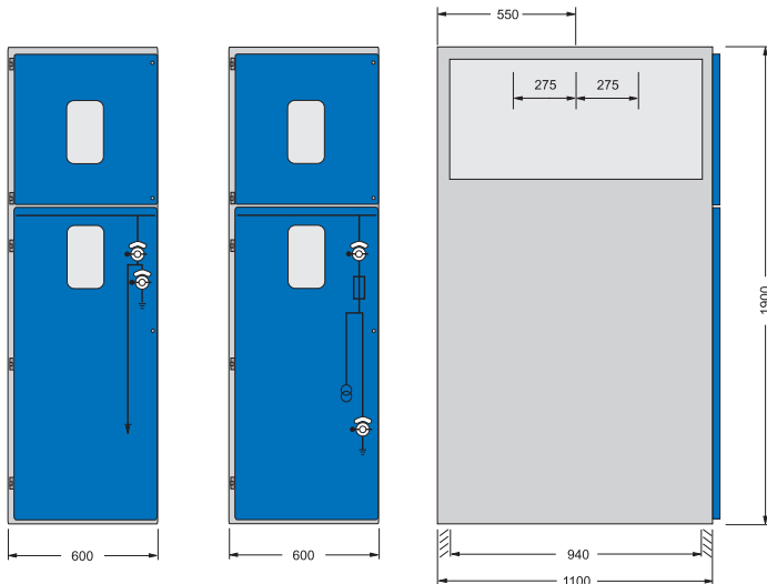
24 kV Switch panel in compliance with drawing HA3-67050
